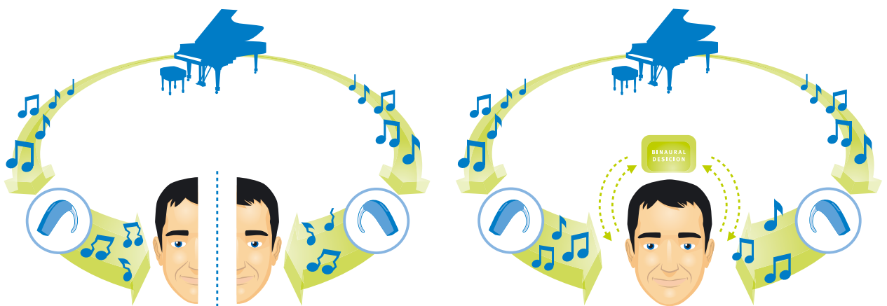
Figure 10: Compared to conventional, independently operating hearing instruments (left figure), Binaural DFC compares the potential feedback signals at both ears before initiating cancellation (right figure).
